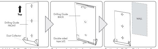
Un-fold the Drilling Guide and open the Dust Collector.
